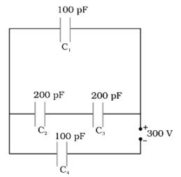
(ii) Obtain the equivalent capacitance of the network shown in figure. For a 300V supply, determine the charge on each capacitor.
